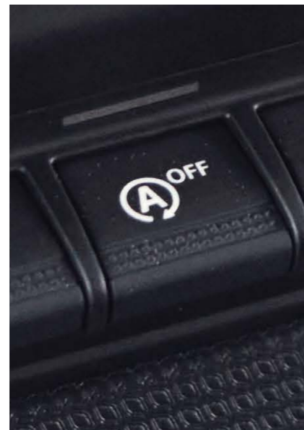
STOP & START SYSTEM standard on all engines.
